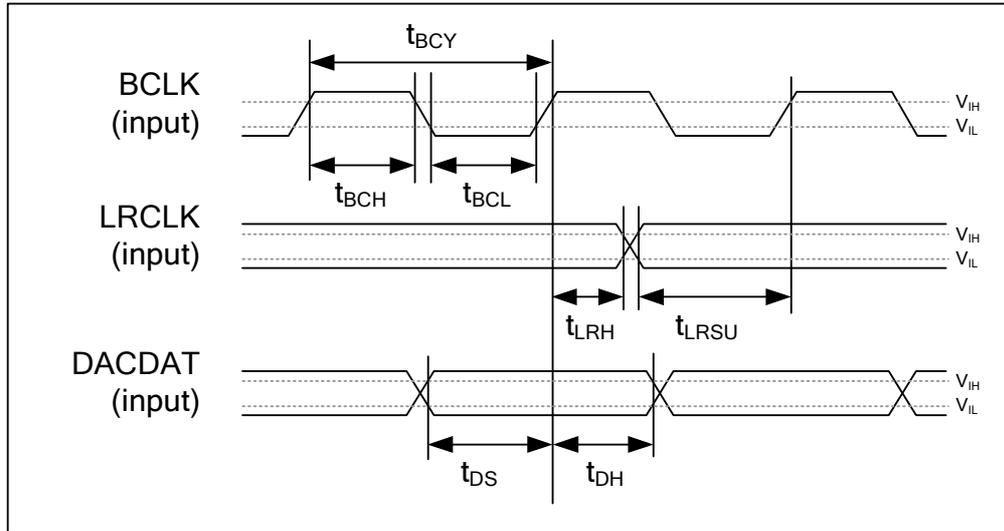
**Figure 2 Digital Audio Data Timing – Slave Mode**
