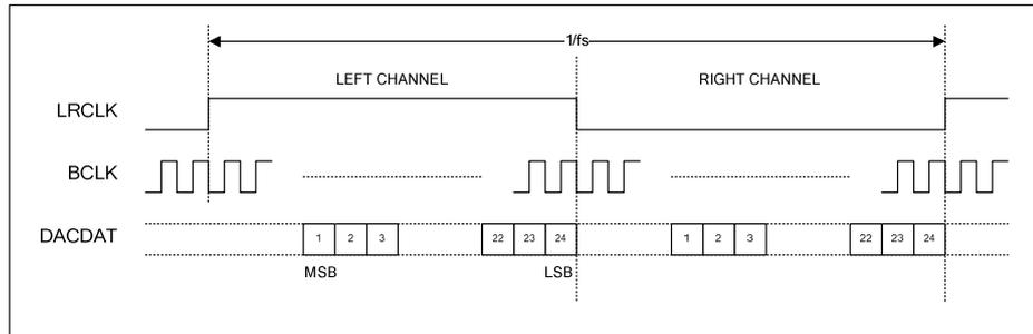
**Figure 6 Right Justified Audio Interface (24-bit word length)**
