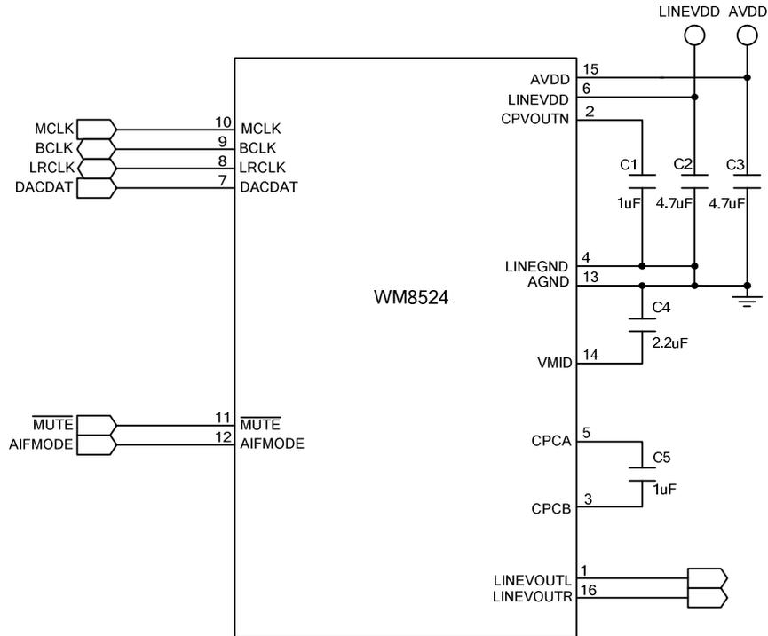
Figure 15 Recommended External Components
