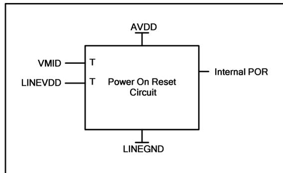
**Figure 3 Internal Power on Reset Circuit Schematic**
