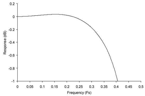
**Figure 14 DAC Digital Filter Ripple – 128fs to 192fs Clock Modes**
