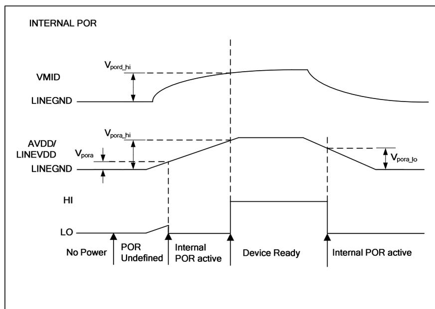
**Figure 4 Typical Power Timing Requirements**
