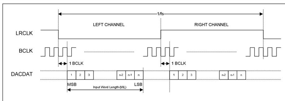
Figure 8 I<sup>2</sup>S Justified Audio Interface (assuming n-bit word length)
